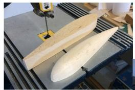
Now that the cowl is pretty much finished, there are a couple other smaller mods I have done. First, the wingtips. The plans just have a simple plywood tip rib which does give a kind of plain square wingtip. I dressed mine up a little bit with some rounded balsa block, hollowed for weight reduction. These wingtip
