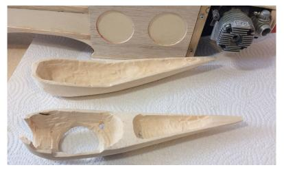
The next step was to position them on the cowl, and mark the spot where the cowl separates from the fuselage. Then cut the cheeks at that spot. Once that's done, glue them on. I glued the front half on the cowl first using 5 minute epoxy, then mounted the cowl on the fuselage so I could properly align the back half.
