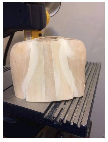
Next I used wood glue to attach the back halves to the fuselage sides. Then some more sanding to get everything smooth. Finally, due to the compound curves all over this cowl and the different parts to make it up, there were gaps requiring filling. Some lightweight spackle to fill the gaps and more sanding.
