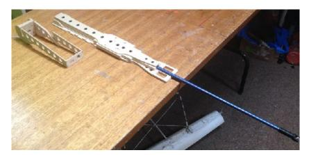
The carbon fiber shaft that is encapsulated by the wood body was roughed up with 120 grit sand paper and c.a'd into place.
